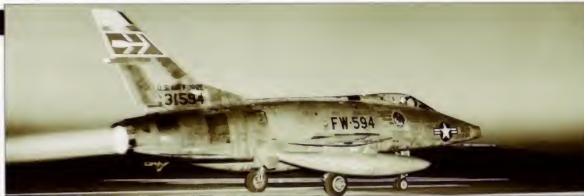
Above: Demonstrating the afterburner fitted to its Pratt & Whitney J57 engine, this F-100 starts its take-off run. Poor fuel economy resulted in the aircraft carrying underwing fuel tanks.
